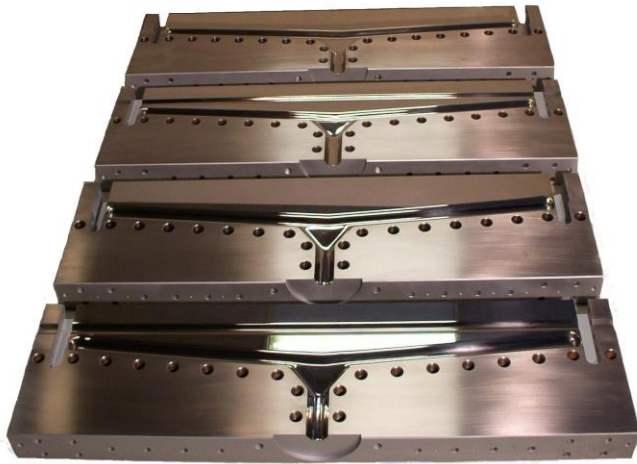
Figure 3. These upper pictures represent the main canal of a coated and non-coated sheet extrusion die (left). These dies processed the same HIPS for 3 years. The right not-coated carbon steel surface is dark and rough. This friction increasing effect notably influenced the plastic flow (stripe formation). The left picture displays a die exposed to similar conditions with a Lunac 1 coating. The improved melt flow as well as surface appearance have not changed since commissioning. Note: The possible bending of the flex lip has to be limited because of the brittleness of Lunac 1 i.e. 0.11% elongation to fracture. Flat die plating can be critical.
