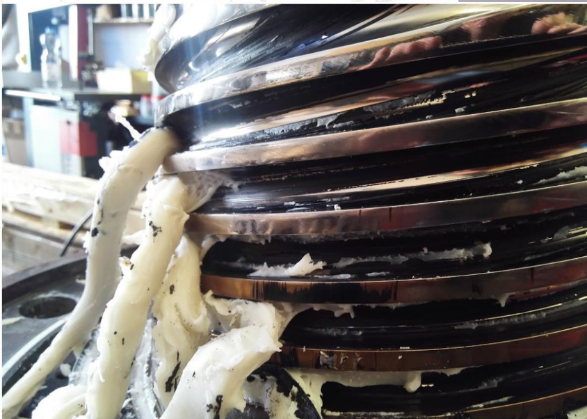
Spiral extrusion die covered with charred plastic (degraded PE). Before Lunac 1 plating the cleaning company needed 2 – 2 1/2 days to restore the original shiny condition of this specific part.
