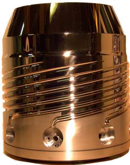
Figure 2. A multilayer die for corrosive PFA plastic processing (at +/- 400 °C/752°F) has completely been plated with 35- 60 μm +/- 2 mil Lunac 1. Only micro-crack free corrosion resistant coatings could resist these conditions. This part was electroless nickel plated before. Electroless nickel tends to form micro-cracks on hardening (hardening takes automatically place starting from 290 °C/554°F. See picture above). On the other hand the electroless nickel coating distribution in the deeper structures is better than the coating distribution of hard chromium or to a lesser extent Lunac. Although the total Lunac-substrate bond is almost unrivalled, the coating itself is rather brittle and consequently care should be taken with respect to the edges.
